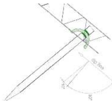
Inclination of T-steel nail
