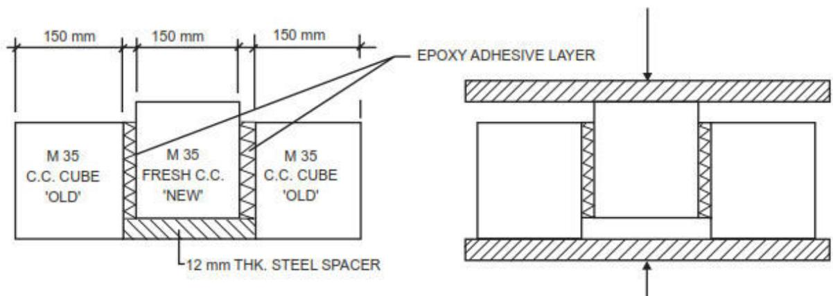
The assembly shall be cured in water for 28 days and steel spacer removed thereafter.
