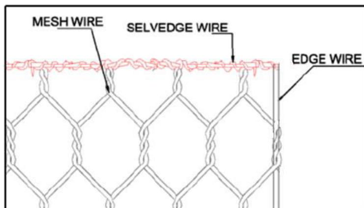
Fig. 24. 4 Mechanically Selvedging and Edge Wire
