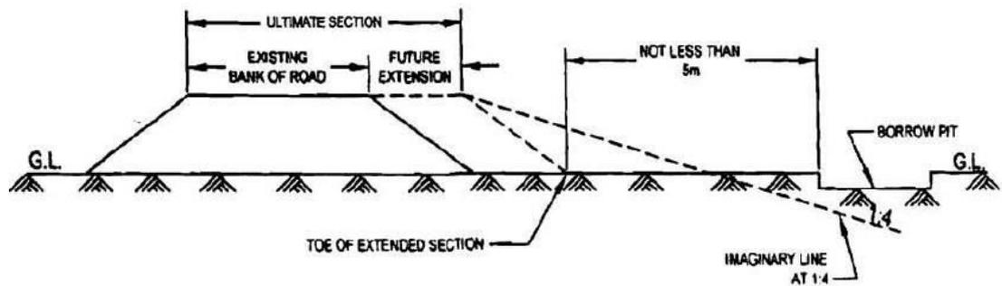
Borrow pits should not be dug continuously. Ridges of not less than 8 m width should be left at intervals not exceeding 300 m. Small drains should be cut through the ridges, if necessary, to facilitate drainage. When it becomes necessary to borrow earth from temporarily acquired cultivable lands, the depth of borrow pits should not exceed 1 m.
