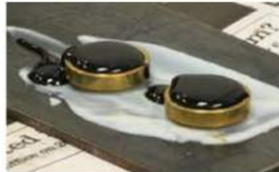
A steel ball is placed upon the bitumen sample and the liquid medium is heated at a rate of  $5^{\circ}\text{C}$  per minute. Temperature is noted when the softened bitumen touches the metal plate which is 25mm below.
