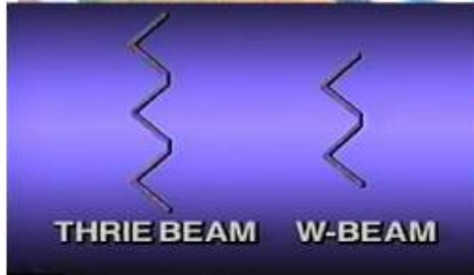
The most common applications for 3 wave or thrie-beam guardrails are bridges on highways , or exit and entrance of tunnels on highways).
